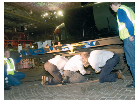
Representatives from the Dutch Government and Railion changing cast iron brake blocks on an SGNS wagon for LL-brake blocks.
